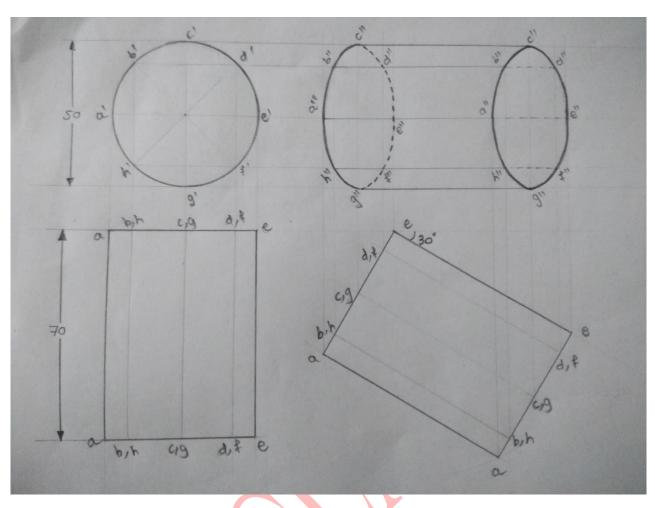
Q.4. (b) Figure Shows three views of an object. Draw its isometric view with 'O' as origin.
